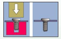
The stud end is fed through a punched or drilled hole and into a lower die. A punch then applies force to the stud. As this occurs, the retaining ring passes through the hole. As pressure is applied, the displacement lobes are seated, forcing the engagement material into the retaining grove.
