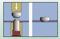
Installation of the STRUX® nut is essentially the same as the STRUX® stud. The retaining ring passes through the hole and as the displacement lobes seat, the engagement material flows into the retaining grove. However, the nut is supported by a spring loaded pin to ensure proper nut alignment. As the nut is staked, the pin retracts.
