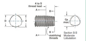
Larger sizes, M6 (#12) and larger, have stabilizing threads to aid alignment and ease starting.
